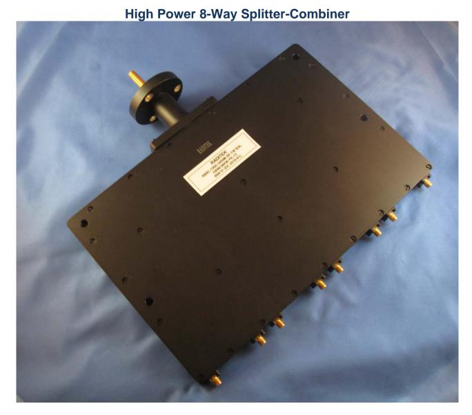
RADITEK'S High Power 8-Way Splitter-Combiner: operates from 1200-1400MHz, Average Input Power 40Watts, 3.5kW Peak, Average Output Power 320Watts, 28Kilo Watts Peak, Isolation: 20 dB min on adjacent ports and 25dB min on non-adjacent ports, SMA Female input Connector, 7/8" EIA output connector.
